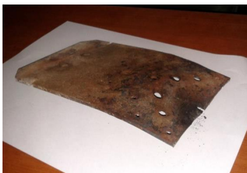
Photo 1 Deformed grate and burned-out burning chamber
